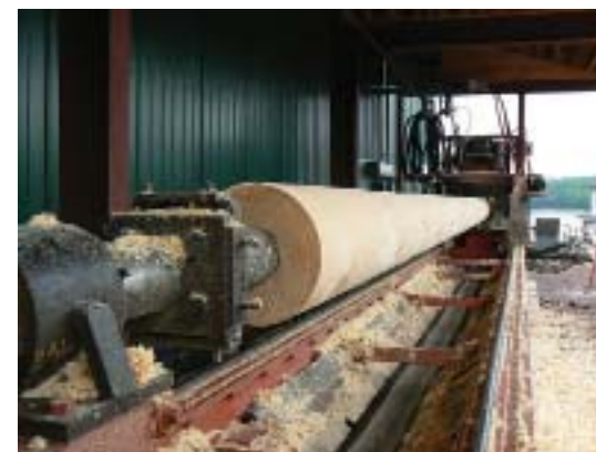
In 2009, Estemerwalt Log Homes unveiled the latest addition to its milling operations, an immense round log lathe that can mill logs with either round or flat profiles to extraordinary lengths and widths. Transporting the machinery took several tractor trailers, and the company had to pour a new foundation prior to its installation to support this massive equipment's weight.
